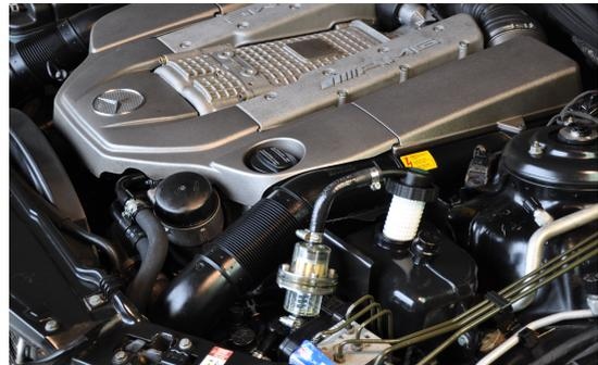
The magnetic filter must be inserted into the black return line leading to the reservoir (black) of the ABC system.
